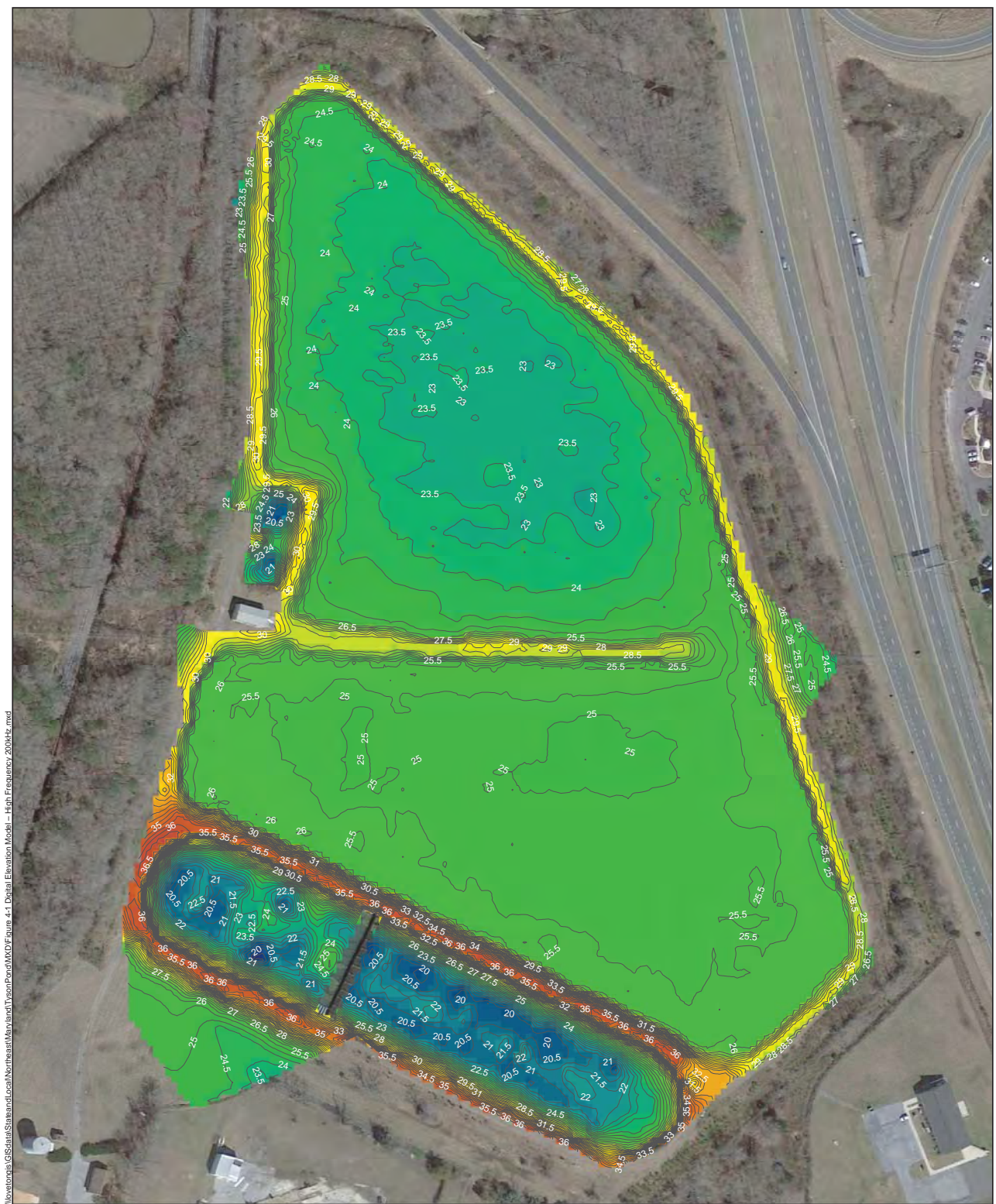
Figure 4-1 Digital Elevation Model – High Frequency (200 kHz) Tyson Lagoon Berlin, Maryland
