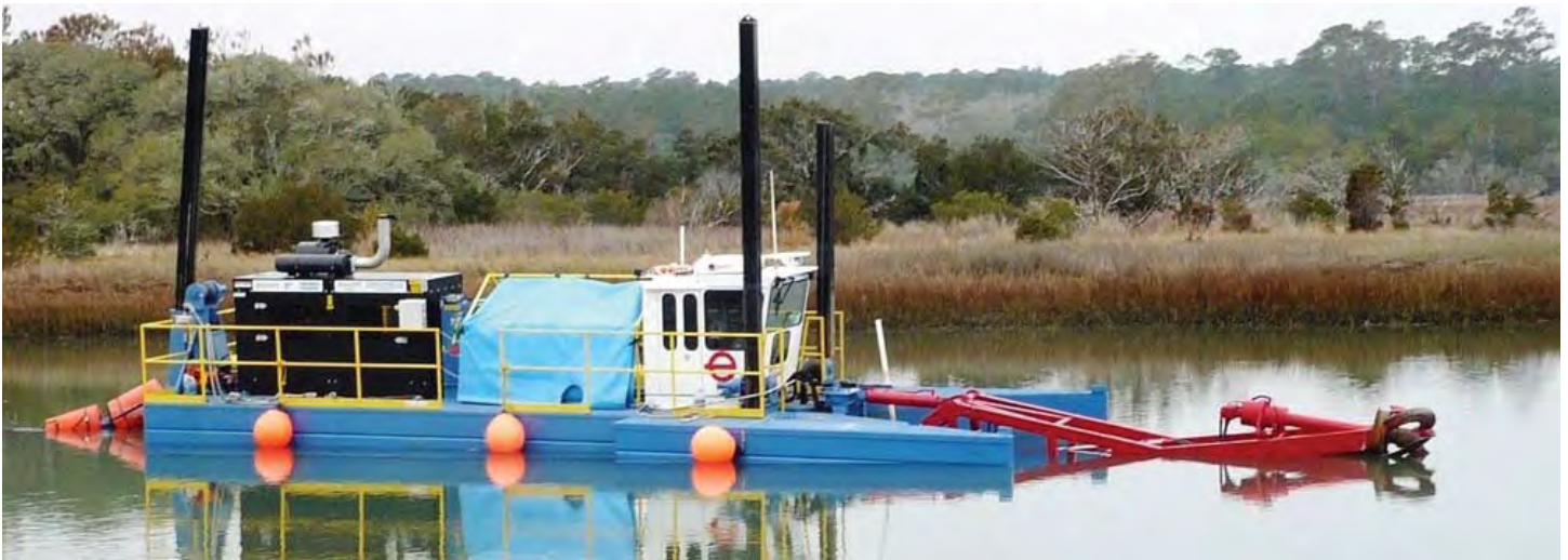
Figure 5-1 Standard Hydraulic Dredge ( http://www.dredge.com )
