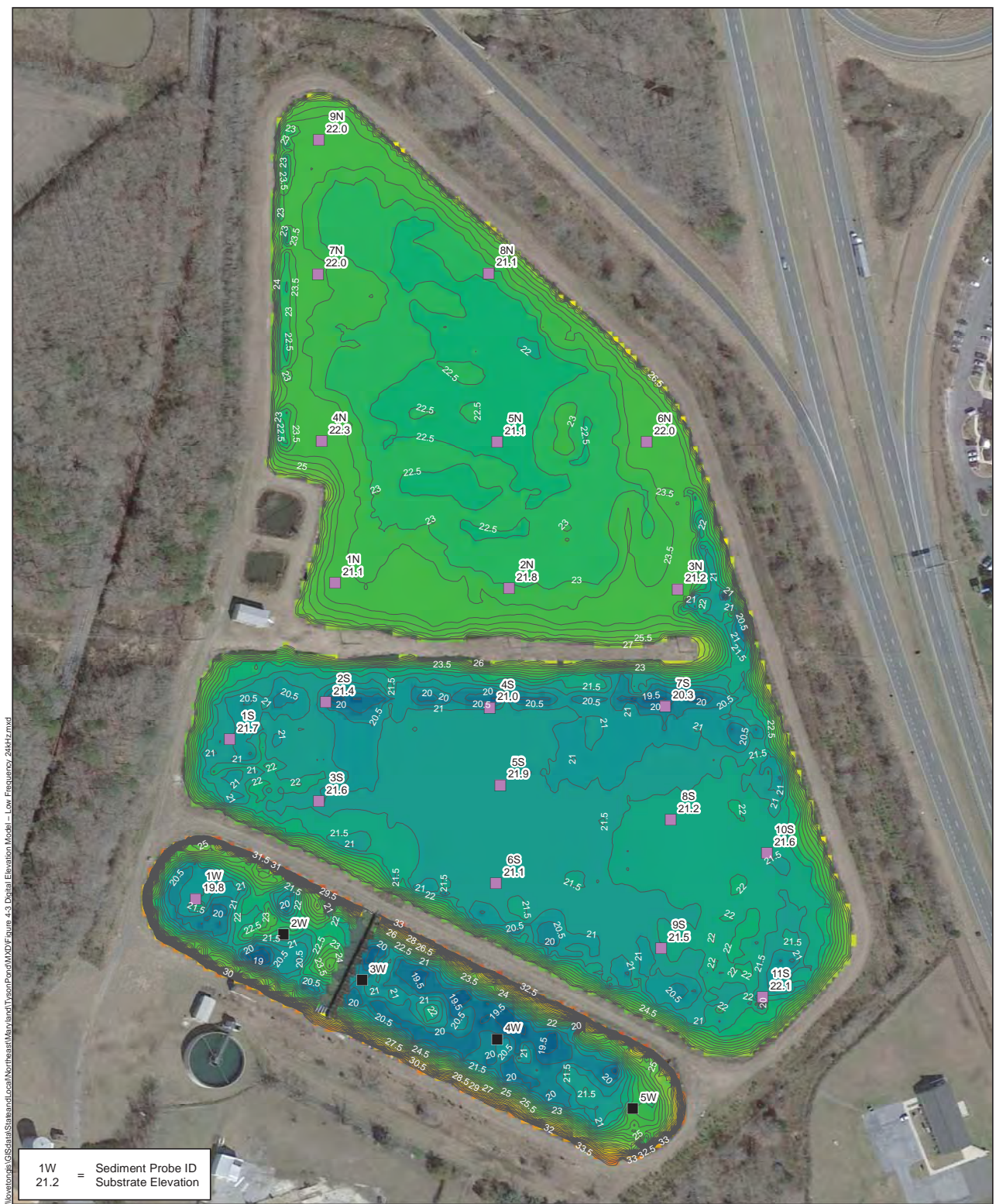
Figure 4-3 Digital Elevation Model - Low Frequency (24 kHz) Tyson Lagoon Berlin, Maryland
